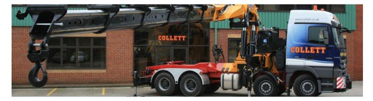
Offering an unrivalled capacity, this latest innovative acquisition offers a powerful weight to ratio performance and utilises 6 boom extensions to provide a maximum reach and lift capacity of 30,000kg at 4.51m and 8,550kg at 15.25m. This hydraulic folding crane is based on a tractor unit with a maximum axle load of 16,500kg and a Gross Vehicle Weight of 150 Tonnes.
