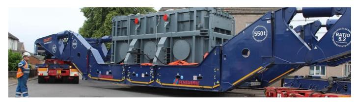
Loaded to a specialist 550 Tonne capacity Scheuerle girder bridge, and accompanied by two heavy tractor units in push/pull formation, the 69.6m long combination travelled the 67 miles from Ellesmere Port to Cellarhead Substation in Stoke-on-Trent.
