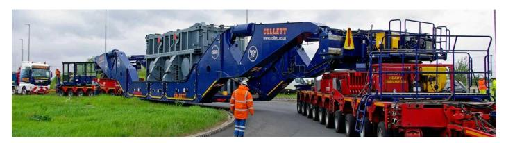
With the transformer arriving at Port Sutton Bridge our Team carried out all port services including stevedoring, lift plans, crane hire and CPA Contract Lift by mobile crane, discharging the 8.6m L x 4.91m W x 4.75m H cargo from the hold of the vessel to our Scheuerle girder bridge.
