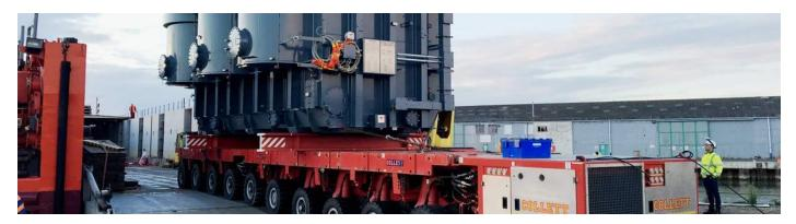
Originating in South Korea the Super Grid Transformer, which measures an impressive 8.7m (L) x 4.9m (W) x 4.7m (H) was scheduled to arrive at the Port of Lowestoft via Rotterdam in late September. With the instruction of the project, on behalf of Hemisphere Freight Services, beginning in June this provided a tight four month timescale in which to plan, execute and complete the delivery.
