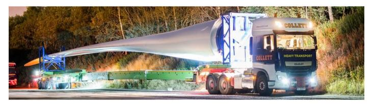
Our Teams undertook the planning and delivery of 494 components including blades, towers, nacelles, drive trains and hubs required for the development of Kype Muir Wind Farm. The 80m hub height towers of the Senvion 3.4MW turbines feature 52m blades, and whilst these are not the largest we've been appointed to handle, they necessitated the use of our Super Wing Carriers due to the problematic road restrictions and alignments en-route.
