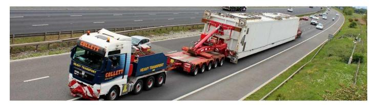
Due to the dimensions of the 4.4m high, 35m long cargo, Collett were required to engineer a bespoke solution to deliver the first, and largest, of the three cargoes.
