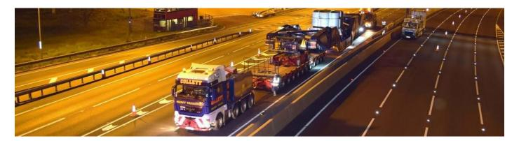
Following a similar successful operation in 2014 which required the relocation of six transformers, the project called upon the expertise of Collett to devise a solution for transporting each of the transformers, measuring 5.08m (H) x 3.5m (W) x 6.5m (L), from Dartford to Drax Power Station near Selby, North Yorkshire. Faced with the task of moving several abnormal loads originating within the busy capital the Collett Team began devising intricate transport arrangements to facilitate the loads.
