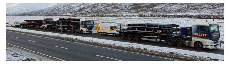
Manufactured at ECS Engineering, the eight gates which would make up the 18.65 Tonne downstream gates and the 13.3 Tonne upstream gates of the Kytra Lock, required transport from Mansfield to Fort Augustus.
