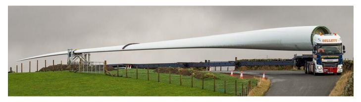
With approval granted for the phase three of Muirhall Wind Farm in South Lanarkshire Collett were called upon to facilitate the import and delivery of eighteen components from the Port of Grangemouth, components which when constructed would form three GE 2.75-120 145m wind turbines.
